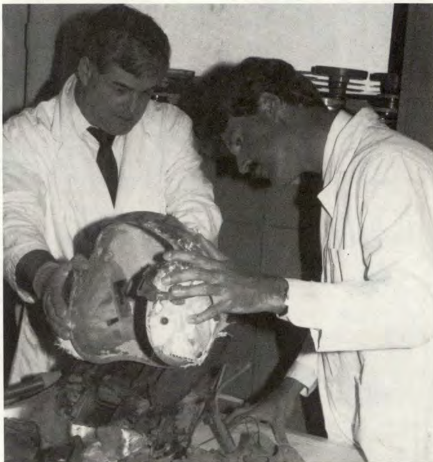
Mike Grost, left, and Perry Nelson work with wreckage from an aircraft mishap to determine what went wrong. This painstaking task is crucial in preventing similar failures in the future.
